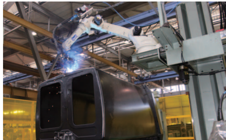
Automatic welding robot for a refuse truck body
