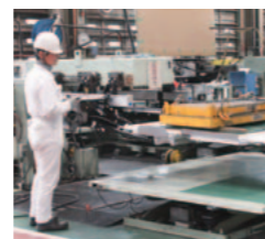
Tailgate lifter load test
