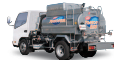
Water truck with aluminum tank
