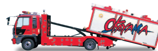
Fire-fighting material transport vehicle Slide type detachable body truck
