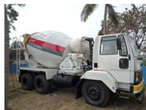
Concrete mixer truck (trial model) manufactured by MKSPV in India
