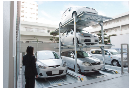
Multi-story parking equipment
