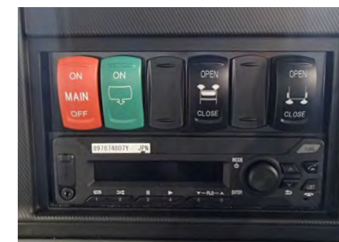
Operation Panel of the Water Sprinkler Truck featuring Pictogram Indicators
