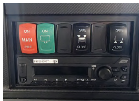
Operation Panel of the Water Sprinkler Truck featuring Pictogram Indicators
