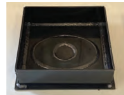
In FY 2024, the challenge was to attach an oval patch to a base plate. At the edges, the welded sections were close together, making it more difficult than the previous year.
