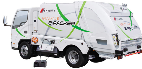
Electric Refuse Truck equipped with power feed system
