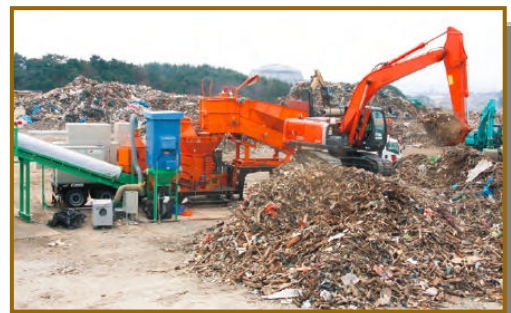
Processing Disaster Waste in Tohoku by "Truck Mounted Pulverizer"
