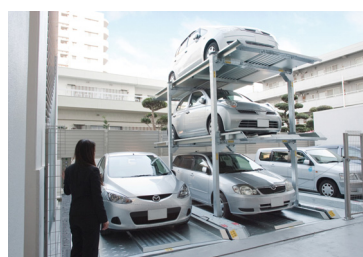
Multi-story parking equipment
