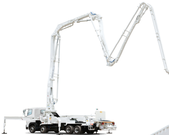
New piston concrete pump truck "PY165-39"
