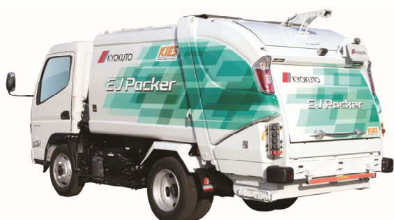
Electric refuse truck for a battery electric vehicle (BEV) chassis
