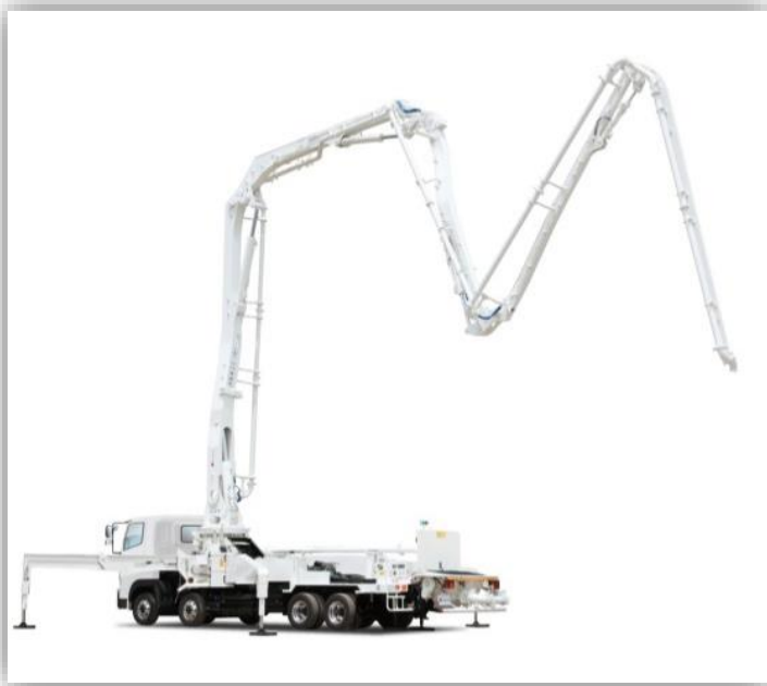
Concrete pump truck (74.4%)
