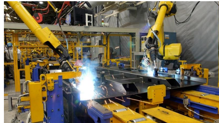
Yokohama Plant Automated line for small dump trucks
