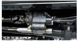
High pressure pump realizes stable discharging operations.
