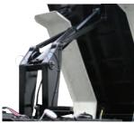
Kyokuto original "GOURIKI™" hoist mechanism realizes high rigidity and stability when dumping and moving.
