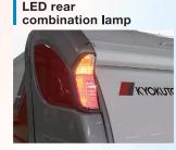
Specially designed LED rear combination lamps have been used as the tail lamps. These improve visibility both from behind and the side, making waste collection work even safer
